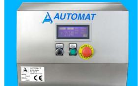
Reference weights can be set manually or automatically. It is sufficient to load a box onto the conveyor belt and press a button which, when the box is weighed indicates the minimum value for reject. This minimum value is also stored in the machine memory.
